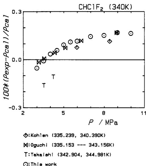
Figure 2. Deviation plots of the density data from the equation of state proposed by Kagawa et al. along the 340 K isotherm.
